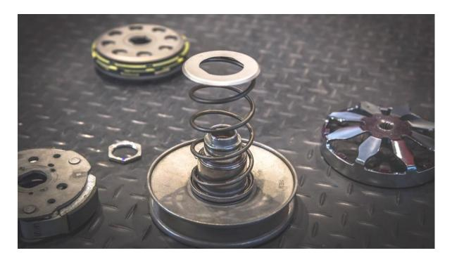
2. First, set the belt in the correct position of the sliding sheave, and then align the two front and rear snap-fit gaps of the clutch plate. The inner edge of the outer edge of the cover is aligned with the clutch notch and placed on the clutch body. Place the whole set on the vehicle. After the tooth is mounted on the pusher and fixed into position, install, and lock the central gear nut.
